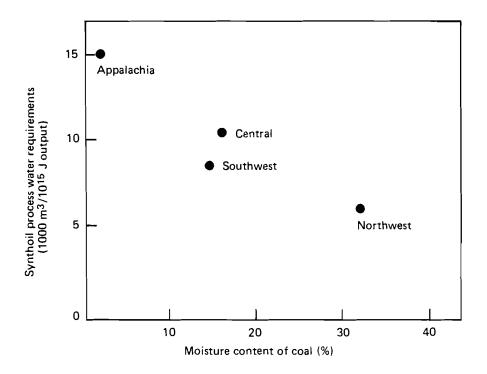
FIGURE C1 Water requirements of the synthoil liquefaction process as a function of the moisture content of US coal. Data from Probstein and Gold (1978).
