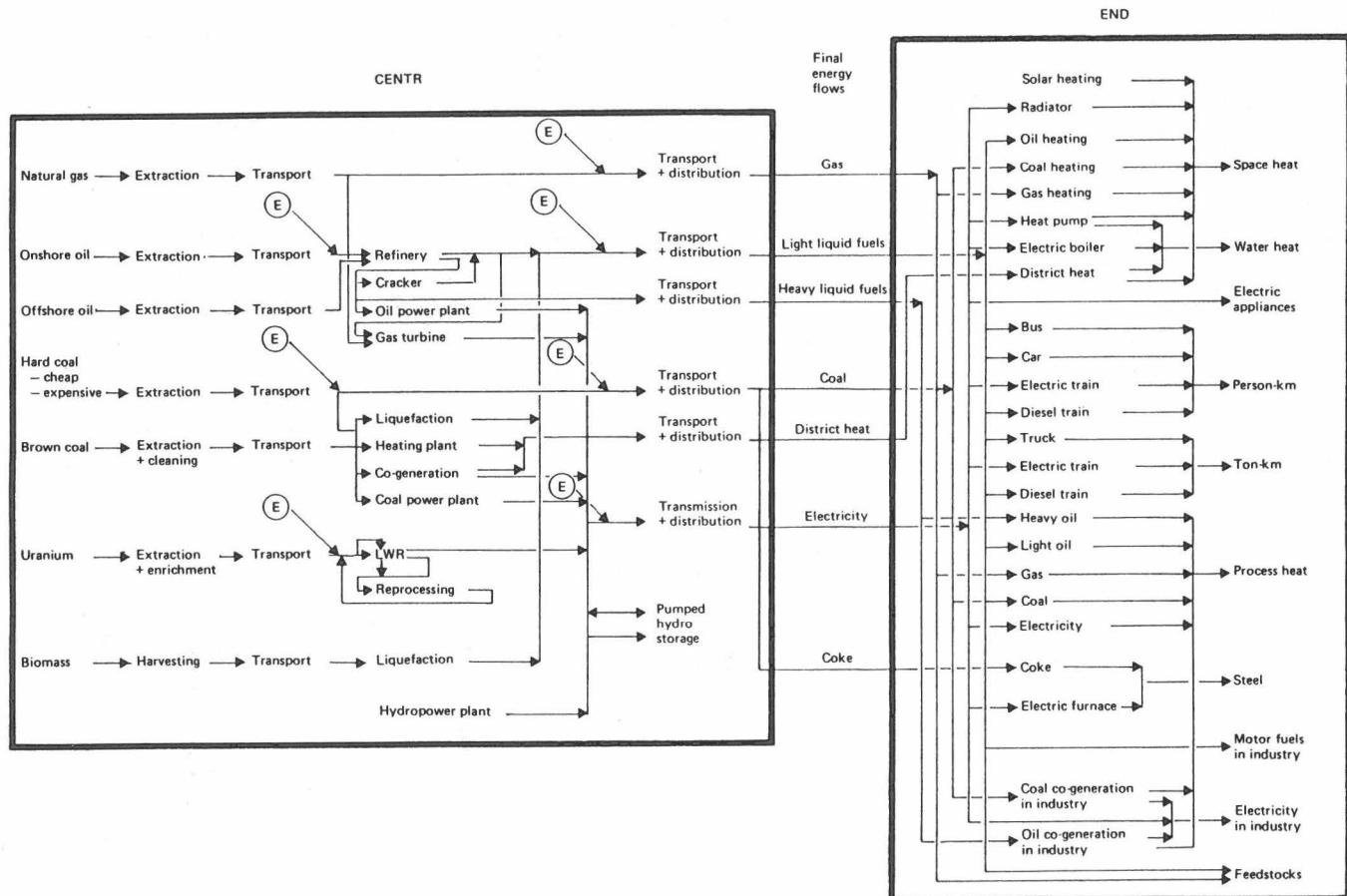
Fig. 1. Structure of the model MESSAGE II.
