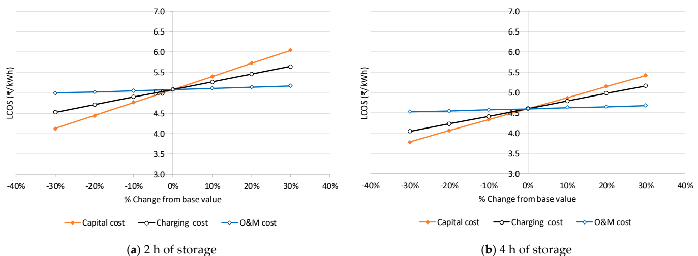
Figure 5. Sensitivity of LCOS to capital cost, charging cost, and O&M cost for (a) 2 h and (b) 4 h BESS configurations.
