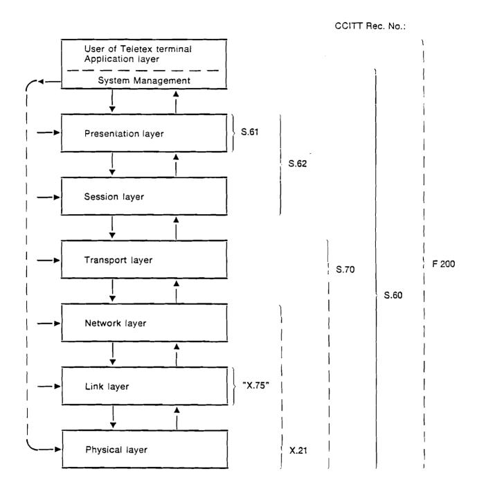
Figure 6. CCITT recommendations relevant to Teletex.
