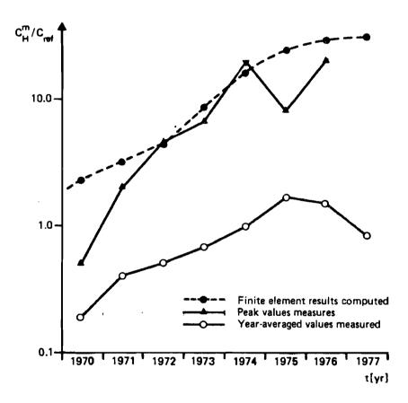
Figure 10. Computed results versus experimental history of contaminant contents in pumped mixing water of SWS during the epignosis period from 1970 to 1977.
