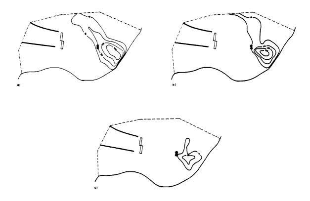
Figure 17. Predicted degradation of contaminant plume by applying two wells (total 2000m<sup>3</sup>/day) starting 1984, under unceasing operating the hydraulic barrier, and with uncontaminated infiltrate ( $C_1^R = 0$  along *efghi*); a) 1985, b) 1995, c) 2015
