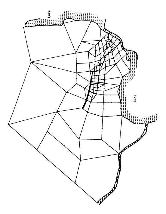
Figure 6. Finite element idealization of study area applied to epignostic modeling (99 elements, 339 nodes).
