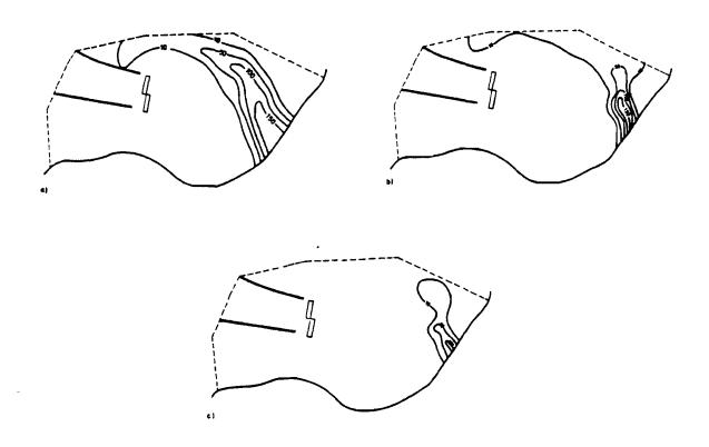
Figure 14. Hypothetical movement of contaminant plume at four-times higher water supply under barrier operating (cut-out of study area) for a) 1988, b) 2027, c) 2060.
