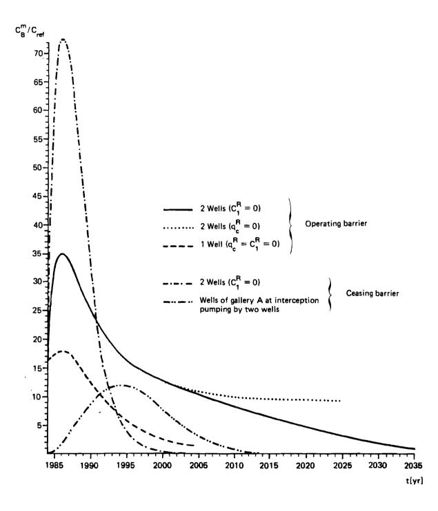
Figure 18. Transient development of normalized well mixing concentration  $C_B^m / C_{ref}$  predicted involving interception pumping the contaminant plume with and without barrier operation.
