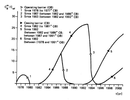
Figure 16. Predicted increase and descent of contaminant content in leading wells of gallery A for variants of intermittent operating the hydraulic barrier (\* up to the end of the year concerned).
