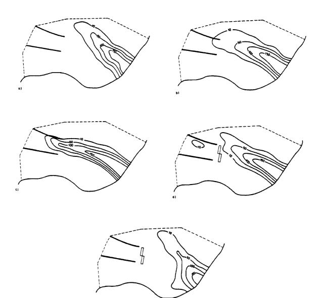
Figure 15. Movement of contaminant plume for intermittent operating of hydraulic barrier (cut-out of study area) at a) 1983, b) 1987, c) 1993, without barrier (since 1982), d) 1995, e) 2003 with barrier (since 1993).
