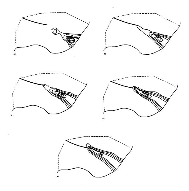
Figure 9. Computed contaminant distribution (cut-out of study area) at a) 1968 (initial field), b) 1970, c) 1972, d) 1974, e) 1977
