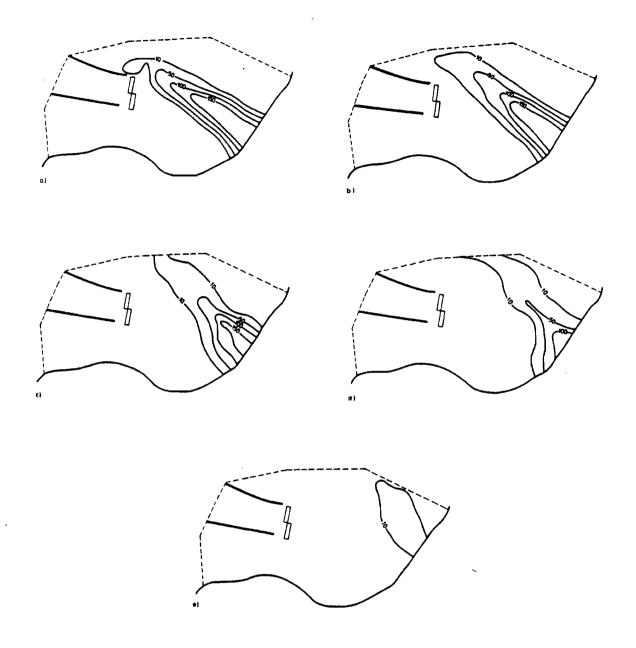
Figure 12. Computed contaminant distribution (cut-out of study area) under permanent operating of phenol barrier for prognosis period in a) 1978, b) 1980, c) 1988, d) 1993, e) 2010.
