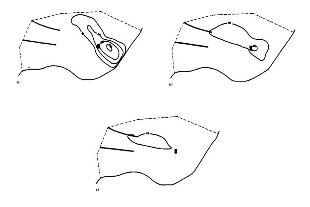
Figure 19. Predicted degradation of contaminant plume by applying two wells (total 2000m<sup>3</sup>/day) with the beginning of the year 1984, under ceasing the hydraulic barrier, and with uncontaminated infiltrate ( $C_1^R = 0$  along eighi); a) 1985, b) 1990, c) 1995.
