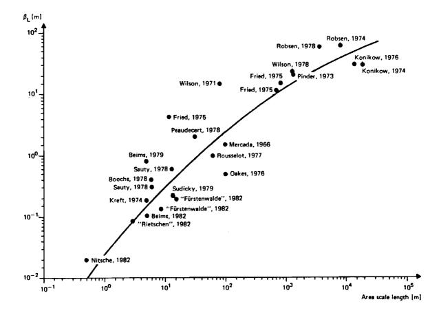
Figure 1. Dependence of longitudinal dispersivity on the area scale length, from Beims (1983)
