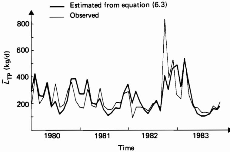
**Figure 6.7.** Validation of the regression model for the Zala River.
