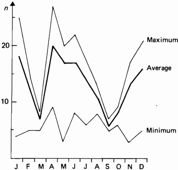
**Figure 6.12.** Number of samples for determining monthly average total P loads (Zala River, 1976–79).
