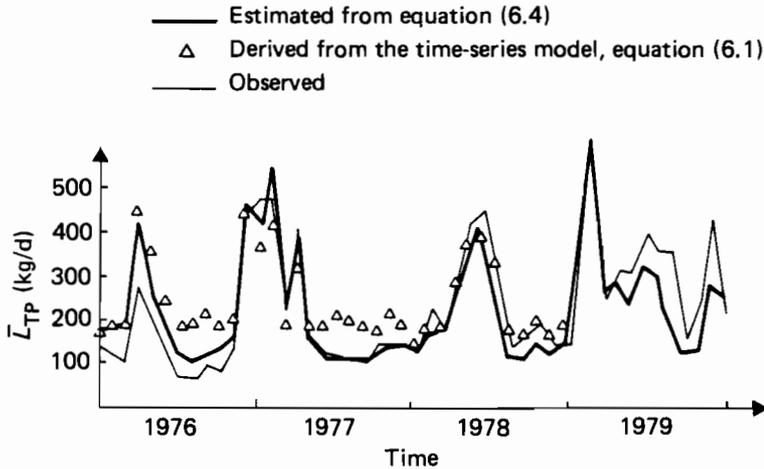
**Figure 6.9.** Comparison of the results of regression and time-series models.
