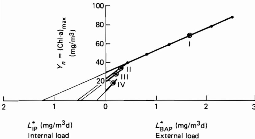
**Figure 4.6.** Aggregated lake eutrophication model: deterministic version.
