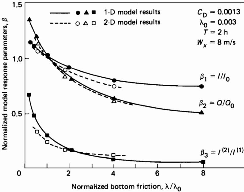
**Figure 9.8.** Summary of model sensitivity to the bottom friction coefficient,  $\lambda$ .
