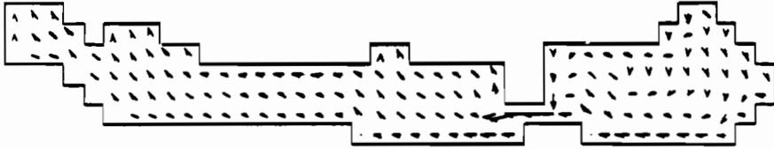
Wind speed = 8.7 m/s      Velocity scale: 15.0 cm/s      Grid spacing = 1900 m
