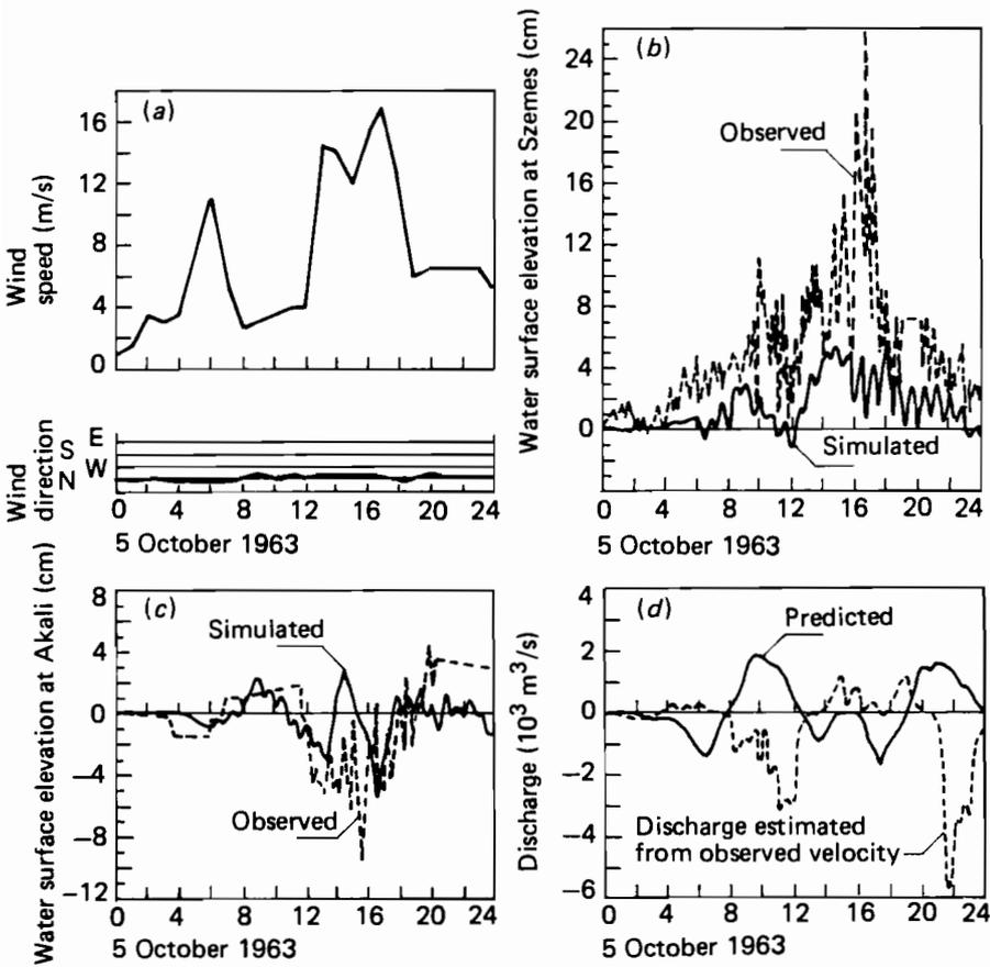
**Figure 9.22.** Comparison of simulation results and observations for the event of 5 October 1963. (a) Wind speed and direction at Szemes; (b) water surface elevation at Szemes; (c) water surface elevation at Akali; (d) current at Tihany.
