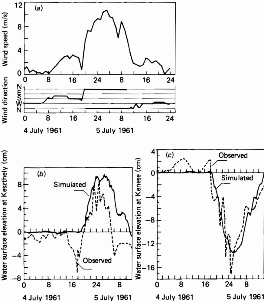
**Figure 9.20.** Comparison of simulation results and observations for the event of 4 and 5 July 1961. (a) Wind speed and direction at Keszthely; (b) water surface elevation at Keszthely; (c) water surface elevation at Kenese.
