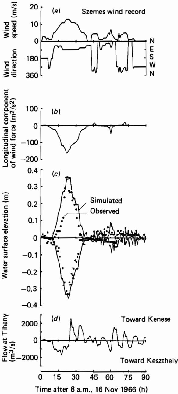
**Figure 9.11.** Comparison of simulation results with observations for the event of 16 November 1966. (a) Wind speed and direction at Szemes; (b) longitudinal component of wind force; (c) water surface elevation at Keszthely and Kenese; (d) flow at Tihany.
