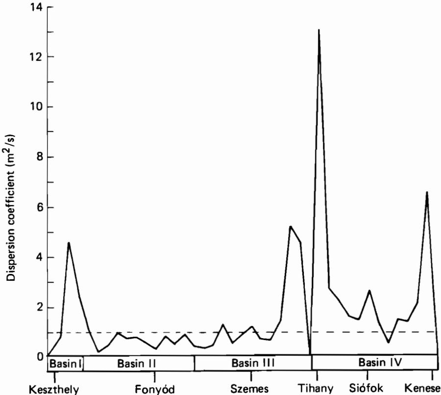
**Figure 9.30.** Spatial distribution of the computed dispersion coefficient averaged over the simulation of July and August 1977.
