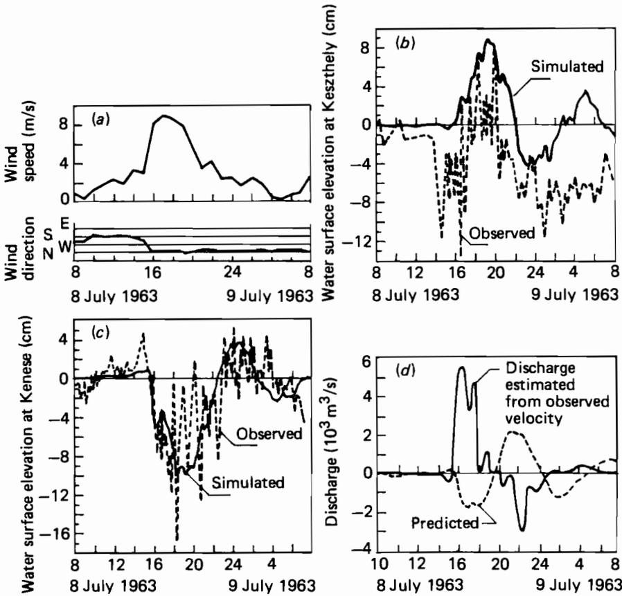
**Figure 9.21.** Comparison of simulation results and observations for the event of 8 and 9 July 1963. (a) Wind speed and direction at Keszthely; (b) water surface elevation at Keszthely; (c) water surface elevation at Kenese; (d) current at Tihany.
