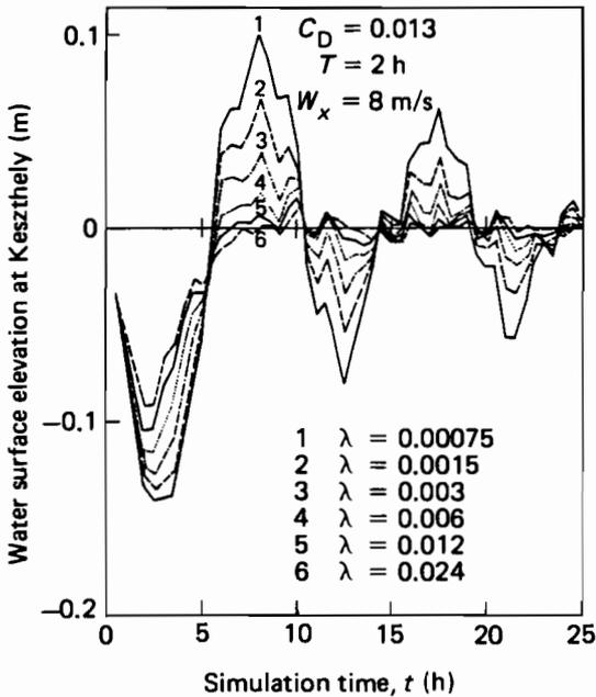
**Figure 9.7.** Histories of water surface elevation at Keszthely showing sensitivity to bottom friction coefficient,  $\lambda$ .
