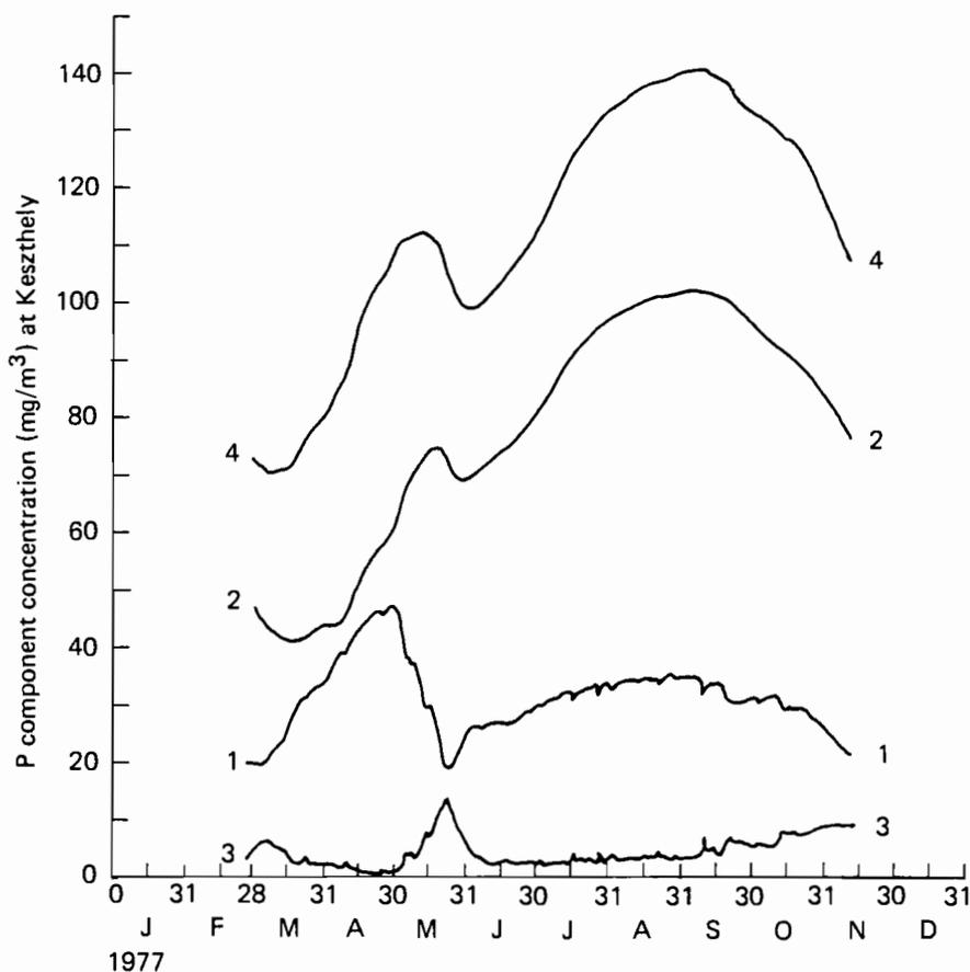
**Figure 10.8.** (c) Effect of model dispersion on predicted P dynamics in Keszthely Bay: with constant dispersion,  $D = 1 \text{ m}^2/\text{s}$ . 1 = total algal P; 2 = detrital P; 3 = dissolved inorganic P; 4 = total P.
