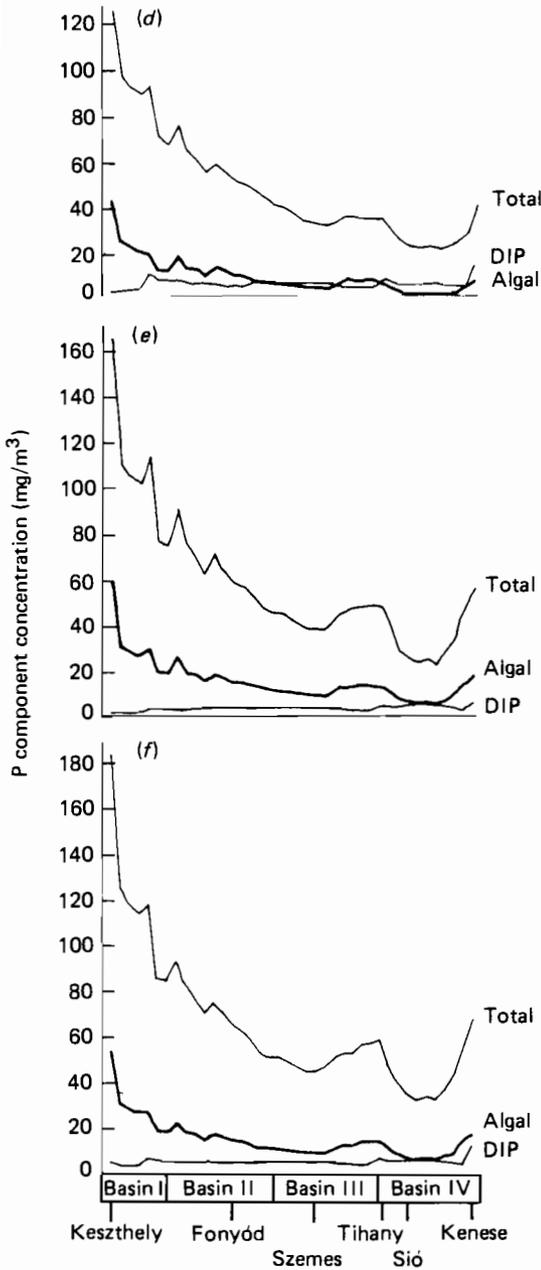
**Figure 10.4** (d)–(f) Spatial distribution of P concentration through time, as predicted by the coupled model base case. (d) 5 June 1977; (e) 5 July 1977; (f) 4 August 1977. Total = total P; DIP = dissolved inorganic P; Algal = total algal P.
