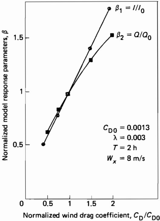
**Figure 9.9.** Summary of model sensitivity to the wind drag coefficient,  $C_D$ .
