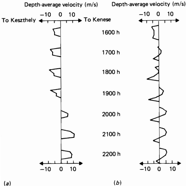
**Figure 9.27.** Lateral velocity profiles predicted in simulation of the event of 8 and 9 July 1963. (a) Model section 18 (between basins II and III); (b) model section 36 (mid-basin IV).
