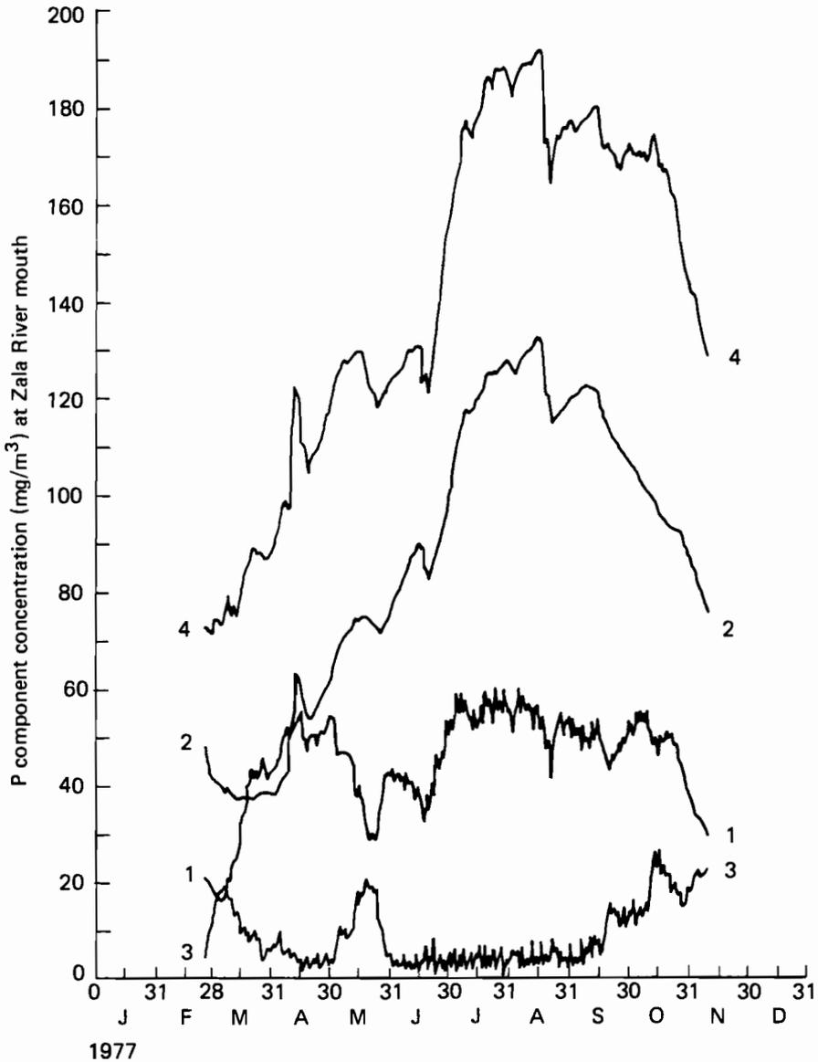
**Figure 10.6.** P dynamics at Zala River mouth predicted by the coupled model base case. 1 = total algal P; 2 = detrital P; 3 = dissolved inorganic P; 4 = total P.
