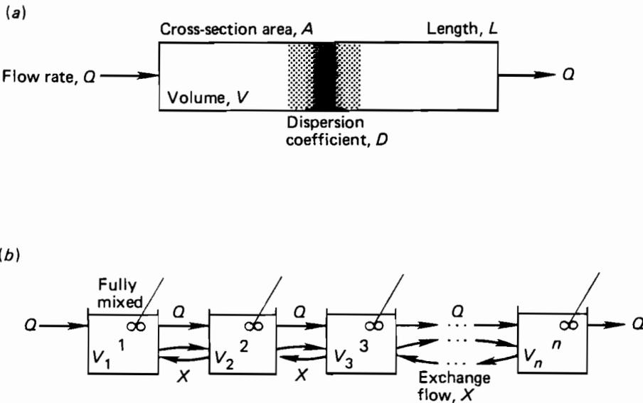
**Figure 10.1.** Schematic representation of conceptual reactors. (a) Dispersed flow reactor; (b) tanks-in-series reactor with exchange flow.
