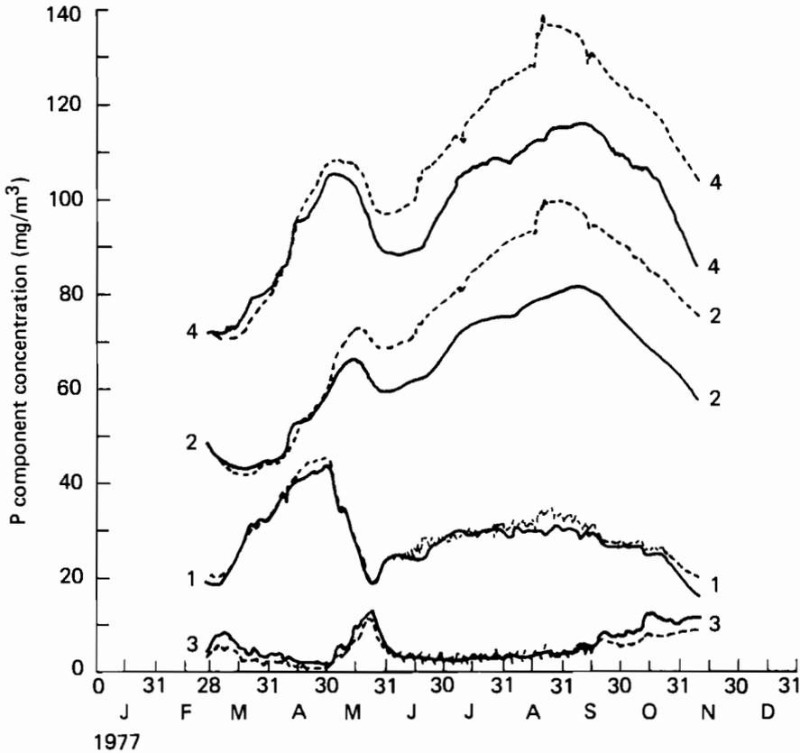
**Figure 10.11.** P dynamics predicted by the four-box model and the coupled model base case. 1 = total algal P; 2 = detrital P; 3 = dissolved inorganic P; 4 = total P. Full line = concentration in basin I predicted by the four-box model; dashed line = concentration in Keszthely Bay (model grid 2) predicted by the coupled definition model.
