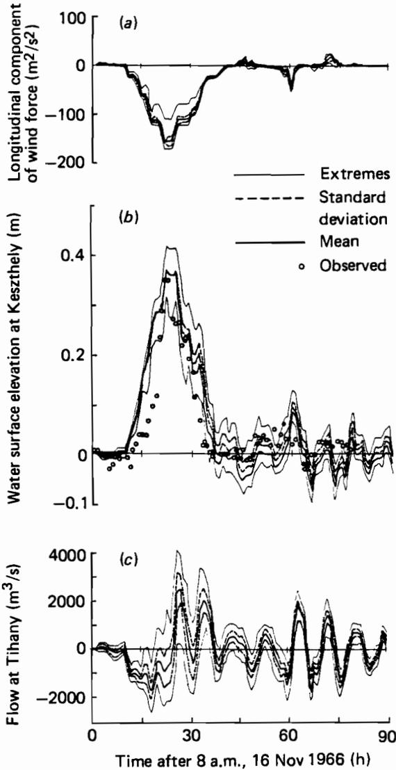
**Figure 9.15.** Monte Carlo simulation of the event of 16 November 1966. (a) Longitudinal component of wind force; (b) water surface elevation at Keszthely; (c) flow at Tihany.
