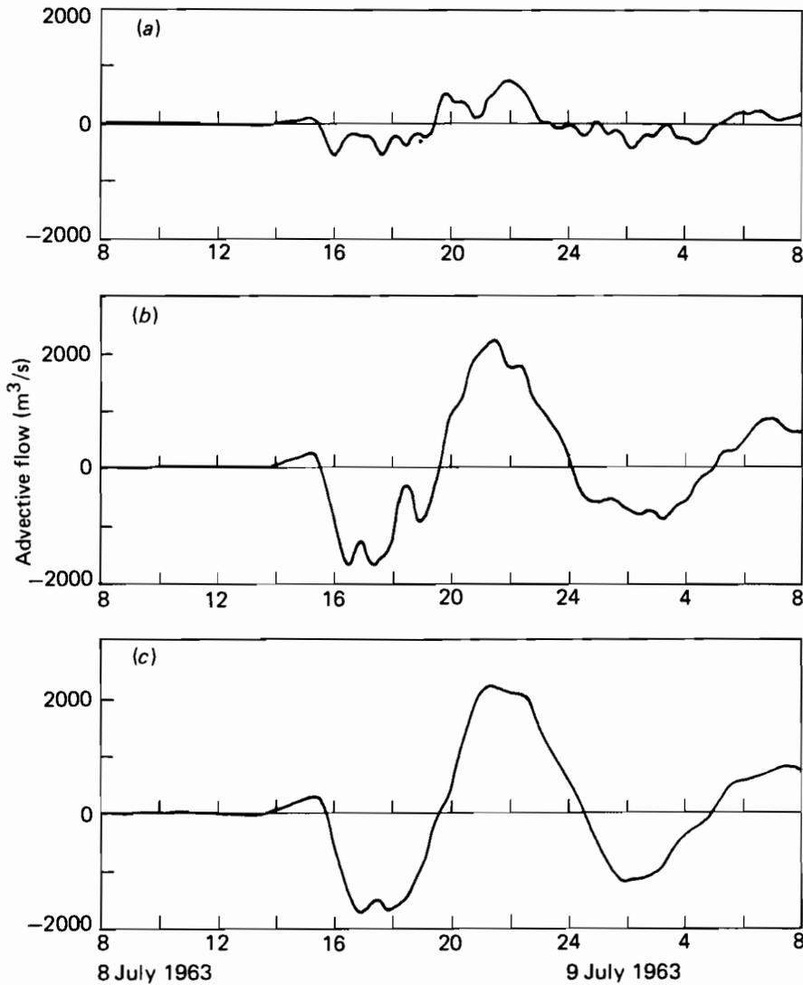
**Figure 9.26.** Advective flow predicted in simulation of the event of 8 and 9 July 1963. (a) Model section 6 (between basins I and II); (b) model section 18 (between basins II and III); (c) model section 29 (between basins III and IV).
