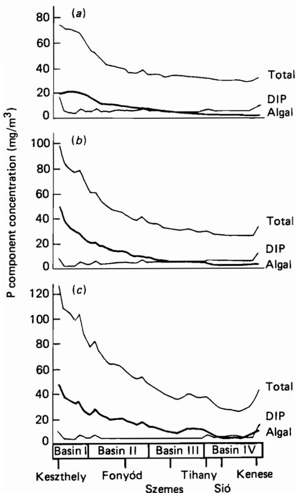
**Figure 10.4.** (a)–(c) Spatial distribution of P concentration through time, as predicted by the coupled model base case. (a) 6 March 1977; (b) 6 April 1977; (c) 6 May 1977. Total = total P; DIP = dissolved inorganic P; Algal = total algal P.
