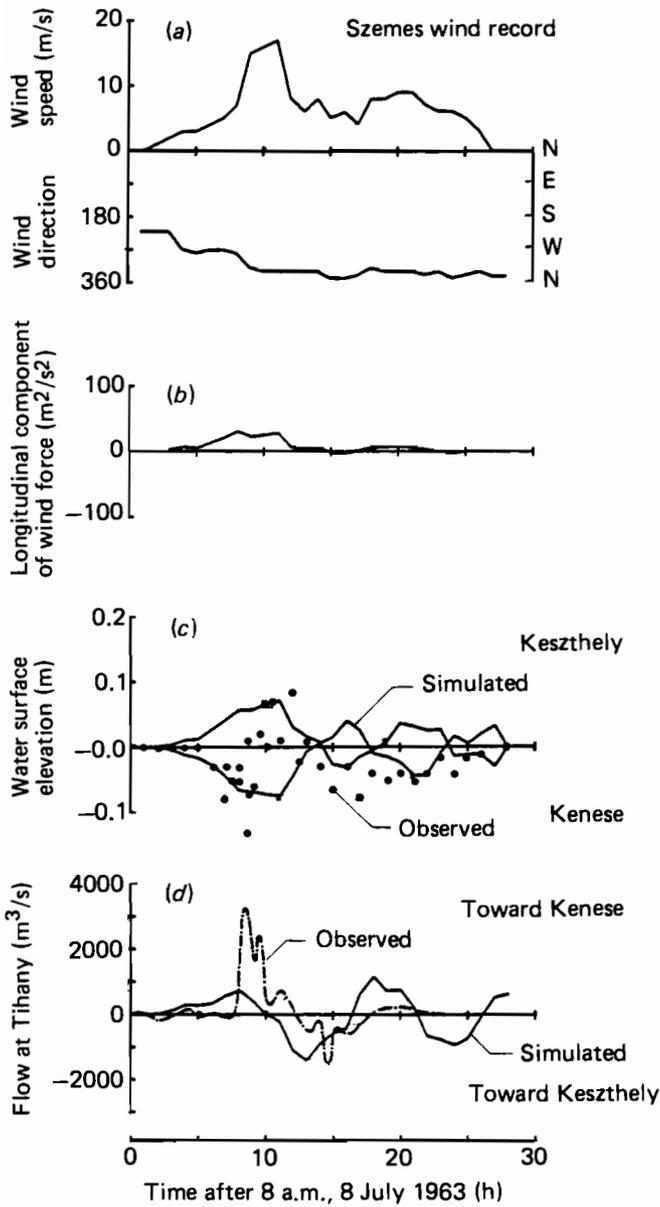
**Figure 9.12.** Comparison of simulation results with observations for the event of 8 July 1963. (a) Wind speed and direction at Szemes; (b) longitudinal component of wind force; (c) water surface elevation at Keszthely and Kenese; (d) flow at Tihany.
