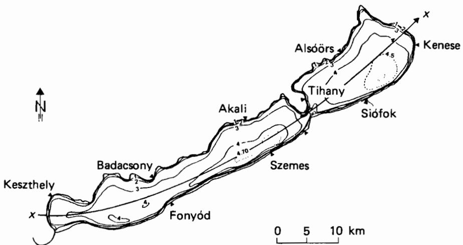
**Figure 9.4.** One-dimensional model coordinate system. Depth contours in meters. Small triangles indicate water surface elevation recording stations.
