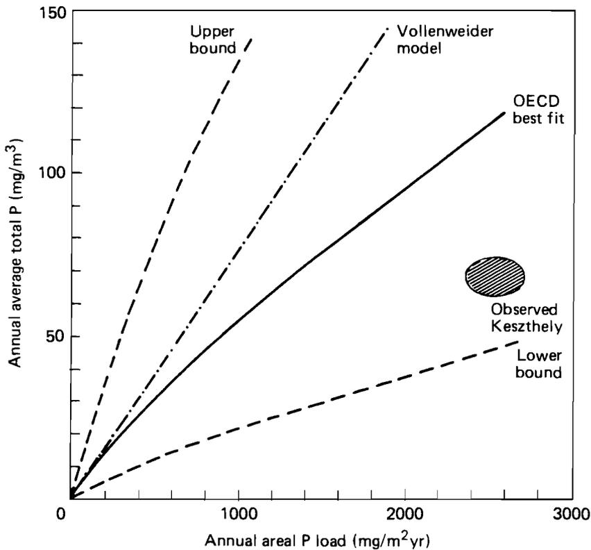
**Figure 3.2.** Relation between annual average total P and areal annual load predicted by OECD for the Keszthely basin, on a linear scale.
