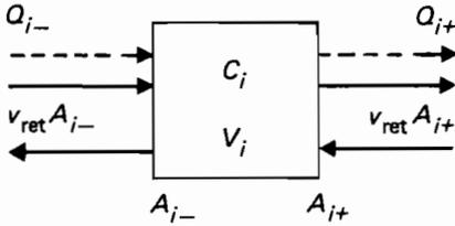
**Figure 11.5.** Exchange rate formulation.  $C$ , concentration;  $V$ , volume;  $Q$ , hydrologic flow rate,  $v_{ret}$ , exchange velocity;  $A$ , cross-sectional surface area.
