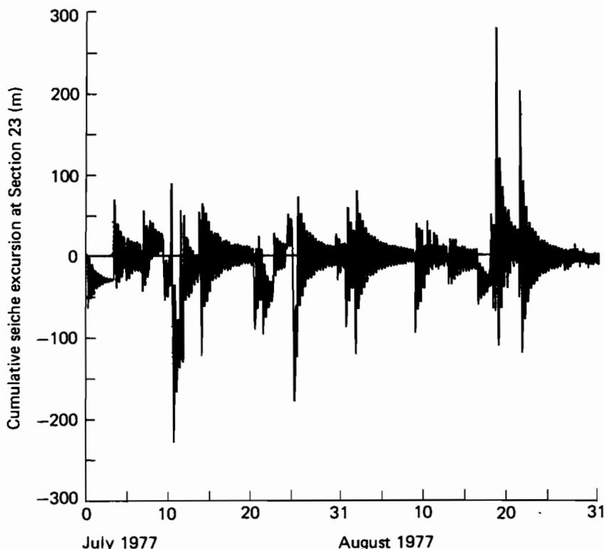
**Figure 9.29.** Longitudinal translation due to seiche advection predicted in the simulation of July and August 1977.
