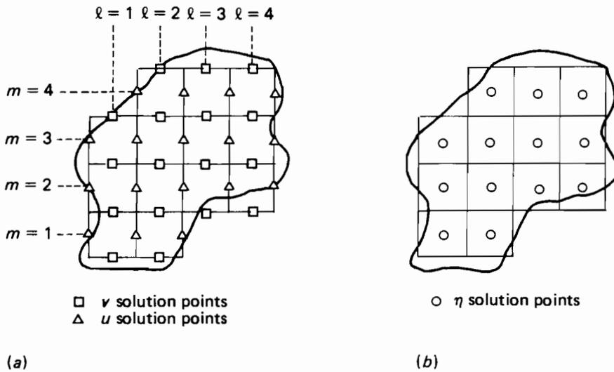
**Figure 9.19.** Finite-difference solution procedure. (a) Full time steps, solution for velocity; (b) half time steps, solution for water surface elevation.
