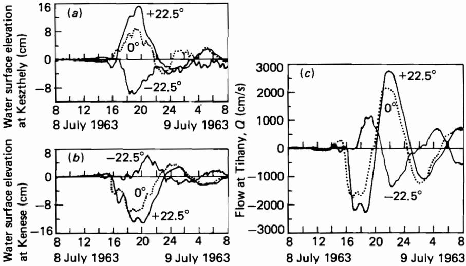
**Figure 9.24.** Effect of wind direction uncertainty on 2-D model simulation results for the event of 8 and 9 July 1963. (a) Water surface elevation at Keszthely; (b) water surface elevation at Kenese; (c) flow at Tihany.
