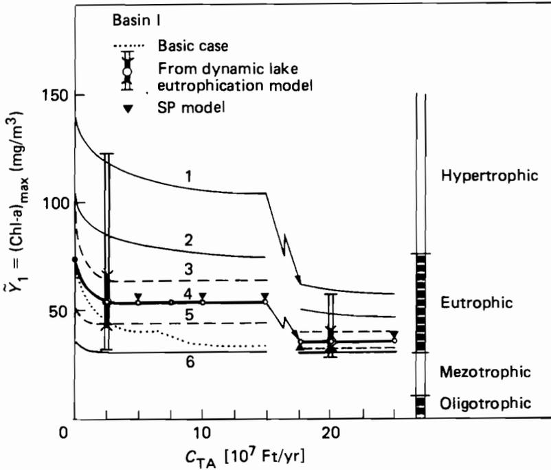
**Figure 4.15.** Solution of the management model for basin I. 4, expectation; 3 and 5,  $\pm$  standard deviation; 2, 95% confidence level; 1 and 6, extremes (all from 1000 Monte Carlo simulations).
