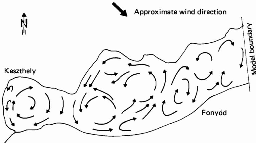
**Figure 9.3.** Qualitative flow pattern observed in Győrke's physical model of western Lake Balaton (from van Straten *et al.* 1979).
