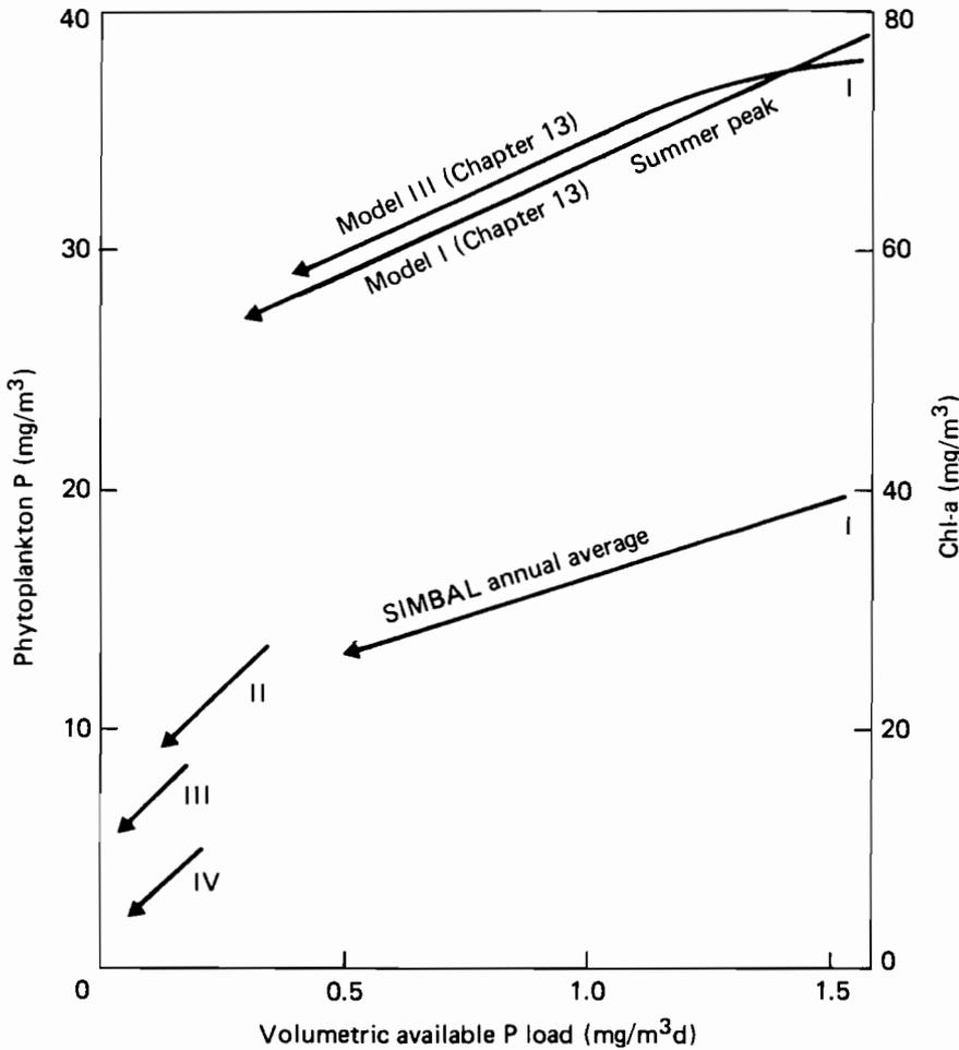
**Figure 3.7.** Phytoplankton concentration response to P load reductions according to SIMBAL (annual average values, all basins) and to models I and III from Chapter 13 (summer peak values, basin I only).
