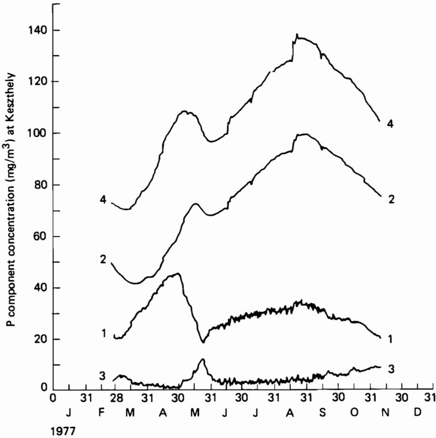
**Figure 10.5.** P dynamics in Keszthely Bay predicted by the coupled model base case. 1 = total algal P; 2 = detrital P; 3 = dissolved inorganic P; 4 = total P.
