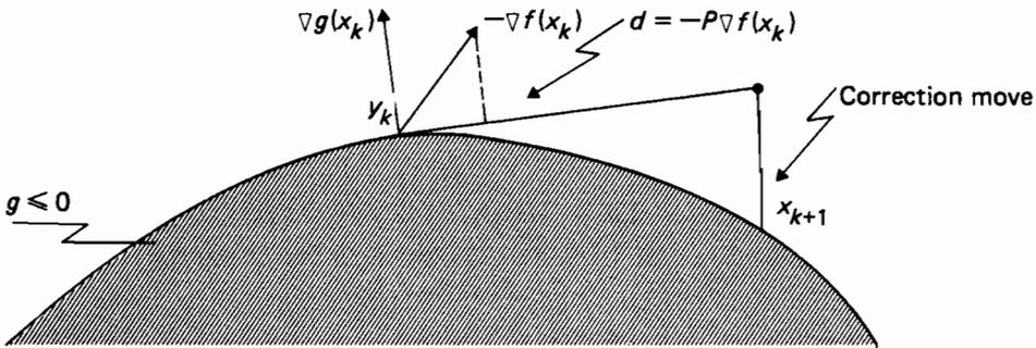
Figure 1 Projected gradient method of Rosen for nonlinear constraints (from Figure 10.5, Bazaraa and Shetty, 1979).
