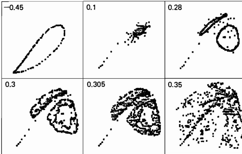
*Figure 4* The value of the next state is plotted against its predecessor: 1000 iterations; the system of Section 3. The parameter  $c$  varies while  $b = -0.45$ ,  $k = 0.0019$ . Magnifications for  $c = 0.305$  and  $c = 0.35$  are depicted in *Figure 7* after  $10^4$ ,  $3 \times 10^4$ , or  $10^5$  iterations.
