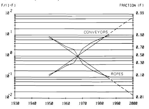
Figure 8B. Share of rope assets and conveyors at inclined workings in underground coal mining industry of the USSR (logarithmic transformation).
