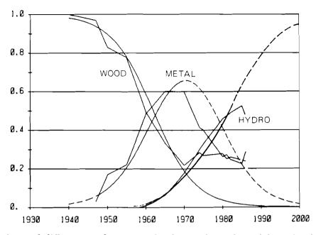
Figure 4A. Share of different roof supports in the total number of faces in the underground coal mining industry of the USSR (linear scale).
