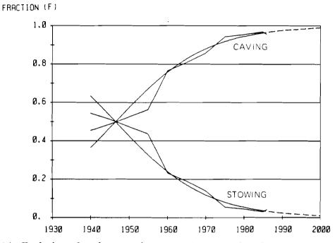
Figure 2A. Evolution of coal output by two main types of roof control in the Donbass (linear scale).
