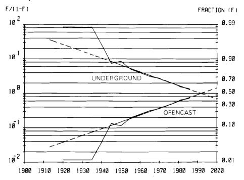
Figure 9B. Share of underground and opencast mining in total coal production of the USSR (logarithmic transformation).
