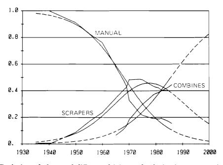
Figure 6A. Evolution of shares of different driving technologies in amount of driving work, total underground coal mining industry of the USSR (linear scale).
