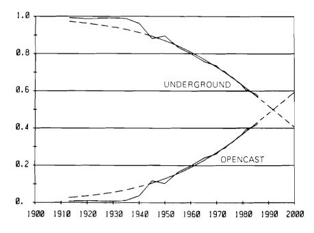
Figure 9A. Share of underground and opencast mining in total coal production of the USSR (linear scale).
