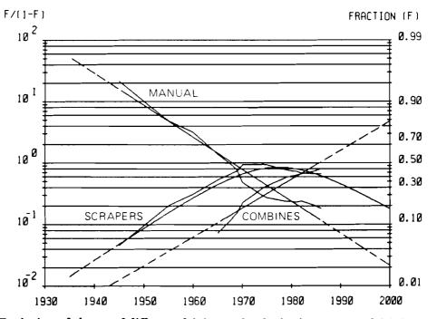
Figure 6B. Evolution of shares of different driving technologies in amount of driving work, total underground coal mining industry of the USSR (logarithmic transformation).
