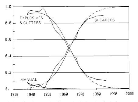
Figure 3A. Evolution of coal output by three technologies of coal winning at coal faces in the underground coal mining industry of the USSR (linear scale).
