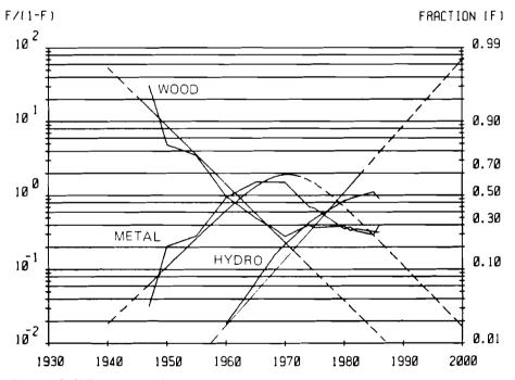
Figure 4B. Share of different roof supports in the total number of faces in the underground coal mining industry of the USSR (logarithmic transformation).
