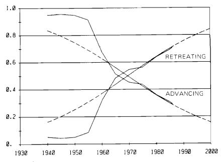
Figure 5A. Share of advancing versus retreating longwall faces in coal output in the Donbass (linear scale).
