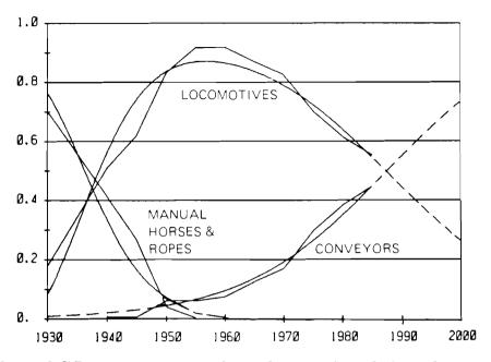
Figure 7A. Share of different transport modes at horizontal roads in underground coal mining industry of the USSR (linear scale).
