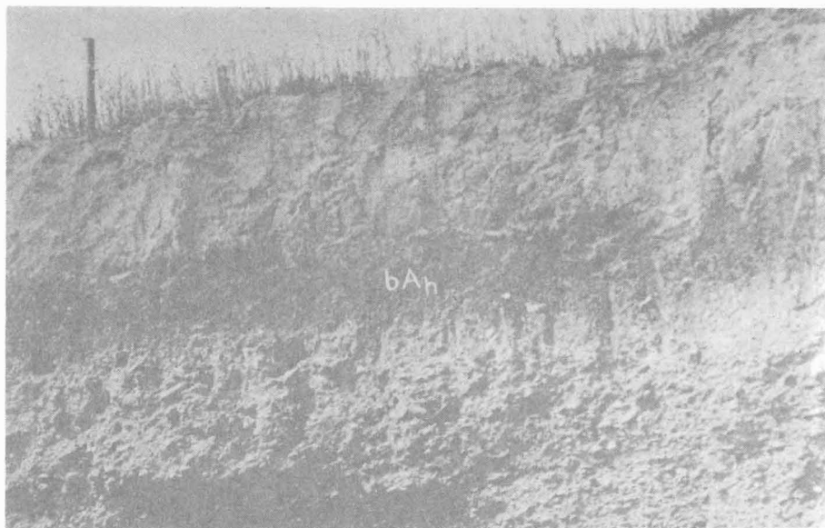
Figure 6. Stollernheim (district of Erfurt), Thuringia, GDR. Gravel-pit exposure at a riverside location. A humus horizon resting on gravel is covered by young Holocene loam-loam deposits of fluvial origin.
