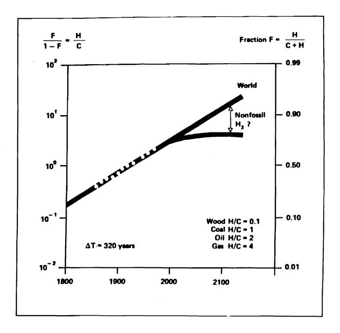
Figure 16. Evolution of the ratio of hydrogen (H) to carbon (C) in the world fuel mix. The figure for wood refers to dry wood suitable for energy generation. If the progression is to continue beyond methane, production of hydrogen fuel without fossil energy or with carbon removal is required (Marchetti, 1985).
