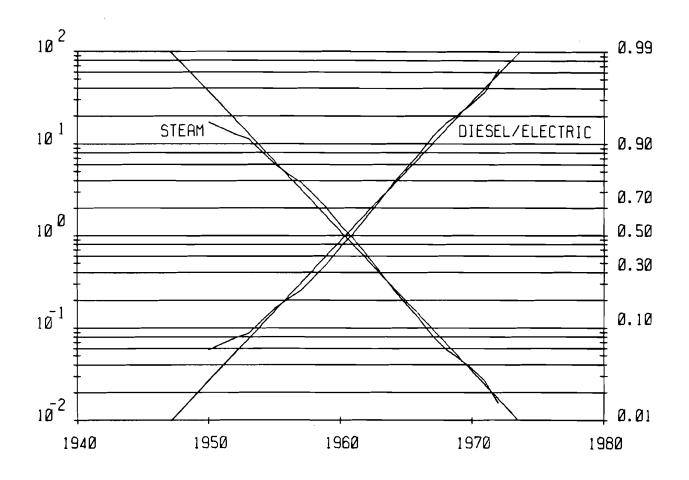
Figure 13. Substitution of steam by diesel and electric locomotives in the USSR. The shares of the two classes of locomotives are given in percent of the total number of locomotives in use. The replacement process lasted about two decades. Similar duration for replacement of the rolling stock and locomotives can also be observed for other countries.
