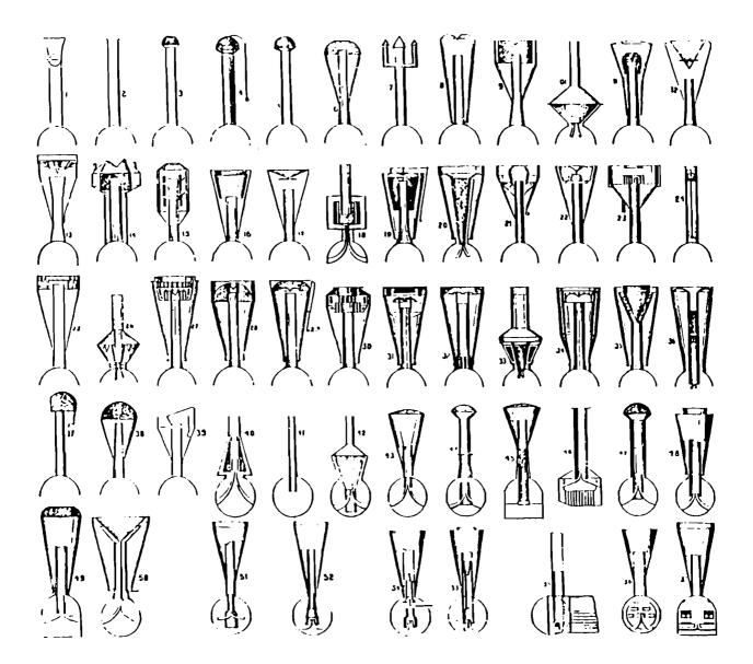
*Figure 5*. Technological variety in response to an environmental and risk hazard: examples of patents for smoke spark arresters for wood burning steam locomotives. Source: Basalla, 1988.
