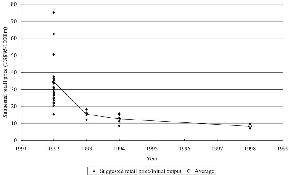
**Figure 4-2:** Price of modular CFL with magnetic ballast.
