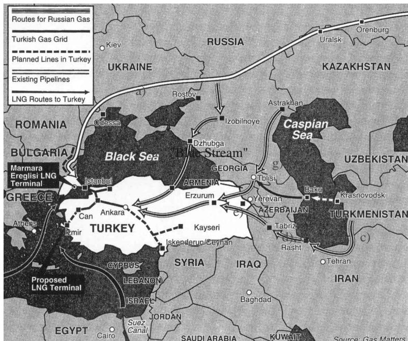
Fig. 6-1. Gas Pipeline Routes to Turkey (Source: Gas Matters).
