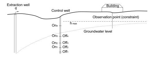
**Figure 17.8.** Scenario for a hybrid control optimization problem PHO in groundwater management. The control well switches the quantity q of the extraction well depending on the switching levels  $On_i$  and  $Off_i$  to maintain an upper limit  $h_{max}$ on the groundwater level.
