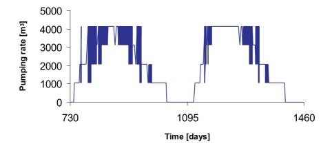
**Figure 17.10.** Pumping rates u(t) (in m<sup>3</sup>/day) of the extraction well using the optimal switching levels as a result of the solution of the hybrid control problem PHO.
