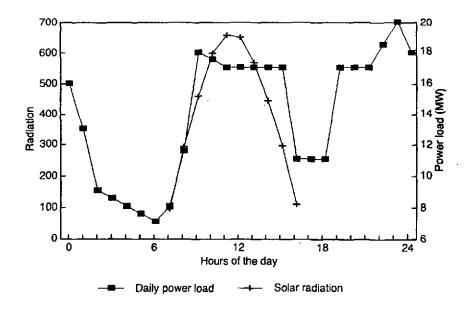
FIG. 2. Solar radiation and power load (January in Tibet).
