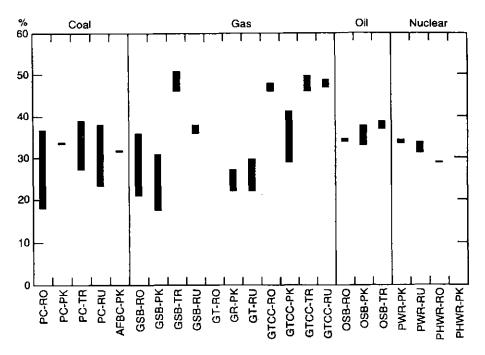
FIG. 8. Preliminary comparison of generating efficiency for CSDB technologies (RO - Romania, PK - Pakistan, TR - Turkey, 'RU - Russia).
