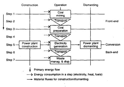
FIG. 3. Schematic representation of a coal fuel chain [3].
