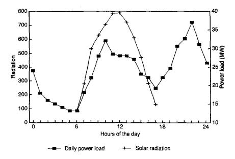
FIG. 1. Solar radiation and power load (July in Tibet).
