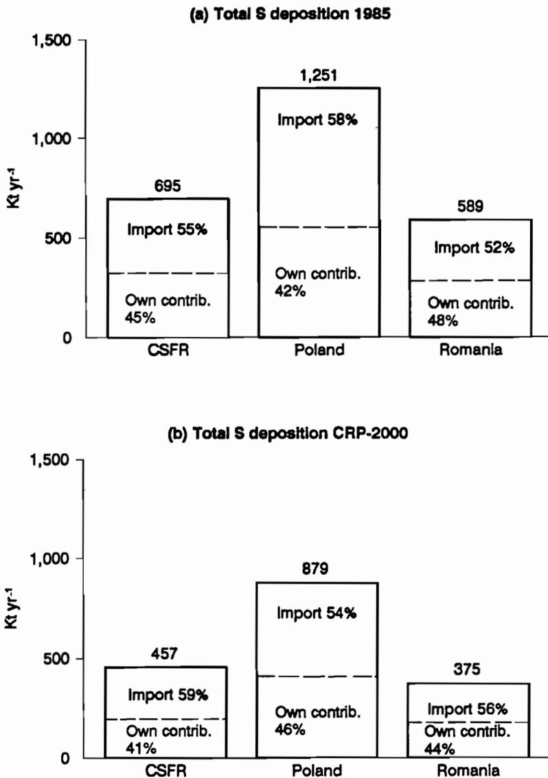
**Figure 6.6.** Budgets of atmospheric loads of sulfur (S) to selected Central and Eastern European countries: (a) 1985 and (b) 2000 under SO<sub>2</sub> Current Reduction Plans (CPR-2000). Sources: Iversen *et al.*, 1989; Alcamo *et al.*, 1990.
