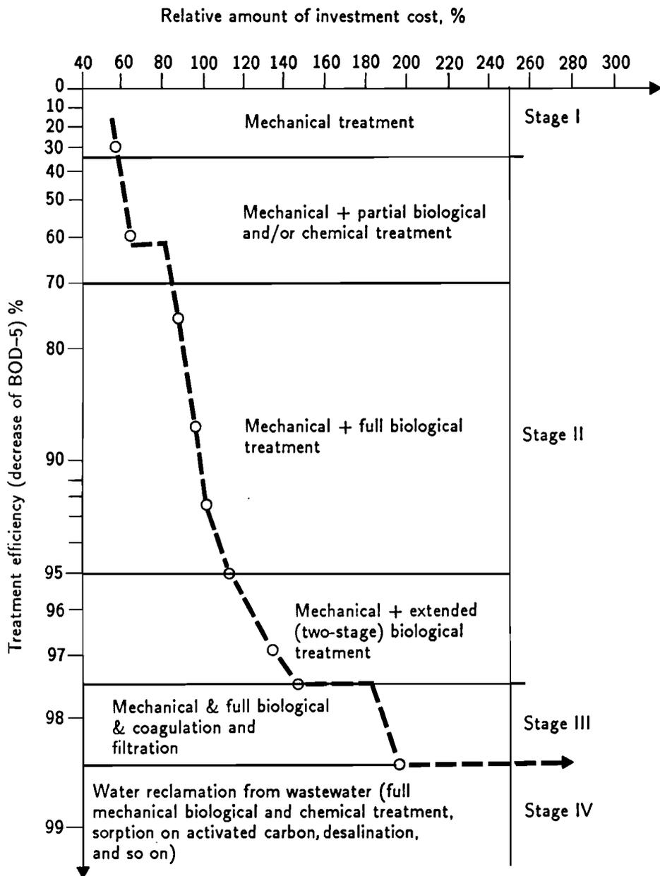
Figure 12.1. Dependence of investment cost of wastewater-treatment plants on treatment efficiency.
