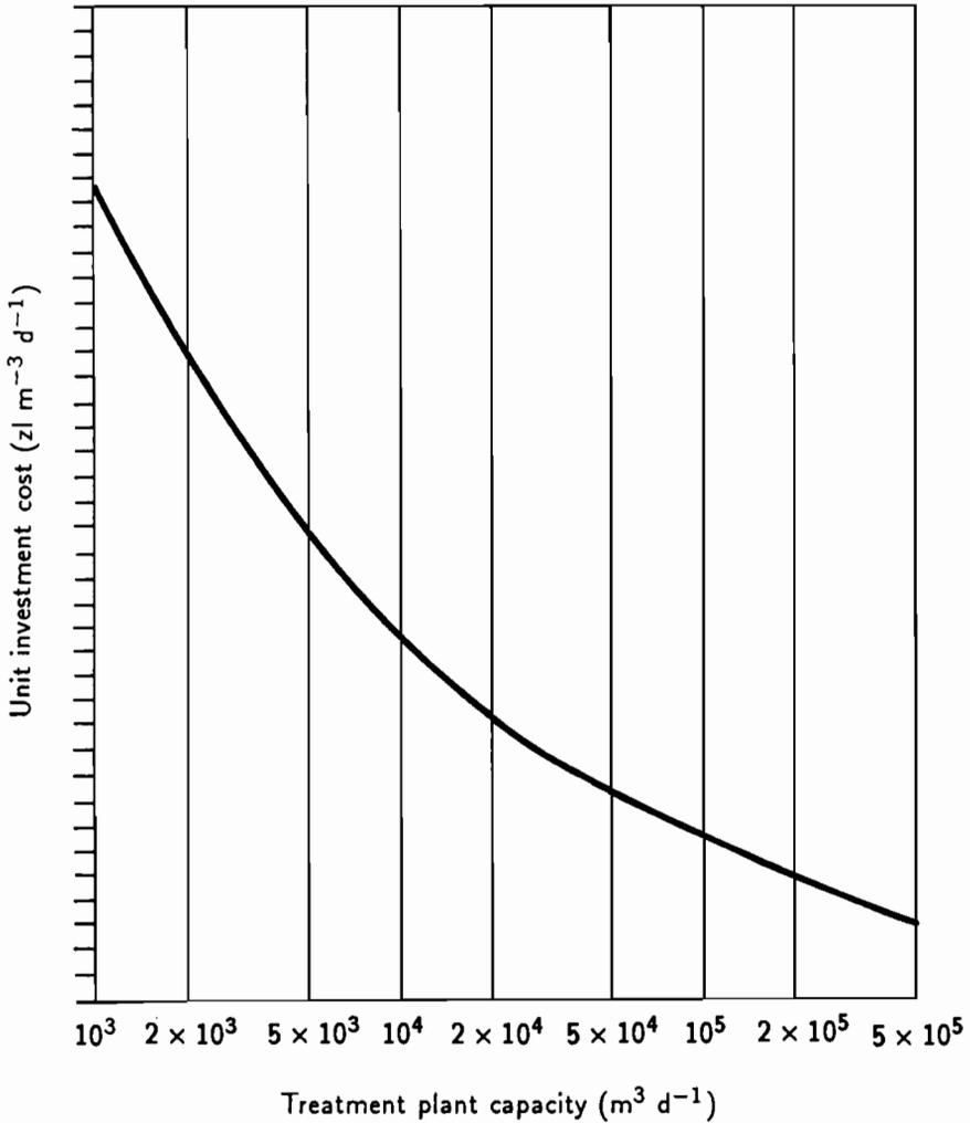
**Figure 12.2.** Dependence of unit investment cost of mechanical-biological wastewater-treatment plants on the capacity of the plants (treatment efficiency decrease of BOD-5 – 92%).
